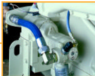
The 150BMGE21RH-6 starters are shown mounted on a Cummins KTA14-M3 and KTA19-M4I.
